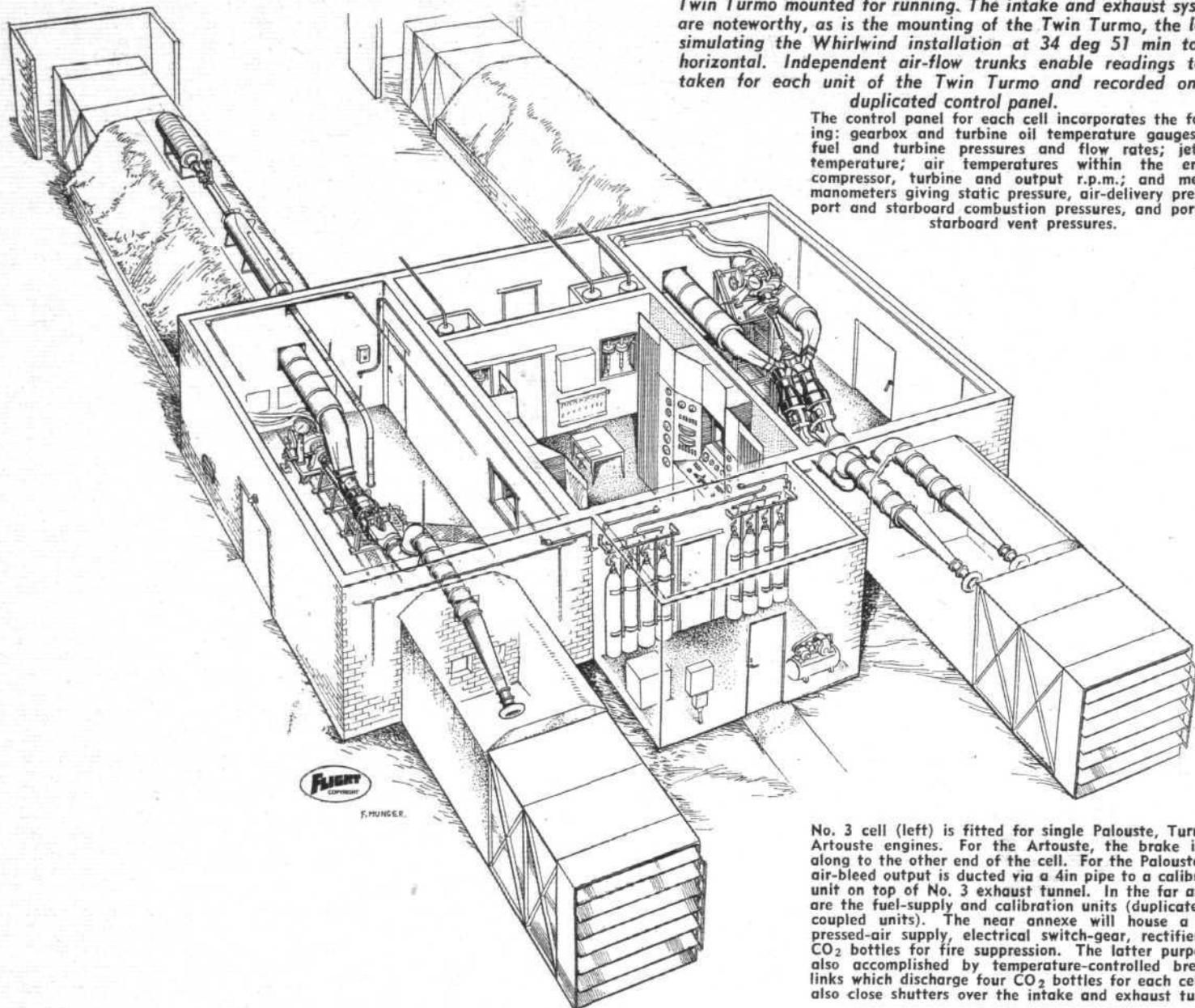
The new twin test house at Brough, showing a Turmo (left) and a Twin Turmo mounted for running. The intake and exhaust systems are noteworthy, as is the mounting of the Twin Turmo, the latter simulating the Whirlwind installation at 34 deg 51 min to the horizontal. Independent air-flow trunks enable readings to be taken for each unit of the Twin Turmo and recorded on the duplicated control panel.
